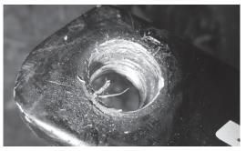
3 INSTALL THE RIGHT HAND PEDAL. This one threads in CLOCKWISE, like a normal screw. Follow the principals as discussed in STEP 2 for the left pedal.
